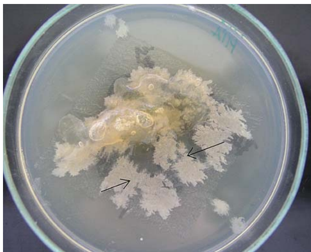
Fig. 1 The utilization of OKCEL ® Mg-T sample by Bacillus licheniformis after 7 days incubation at 30 °C in Nutrient agar no. 2. An arrow indicates the decomposed sample
